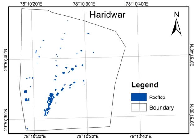
Fig. 6 Rooftops extracted using GIS analysis for usable area calculations
